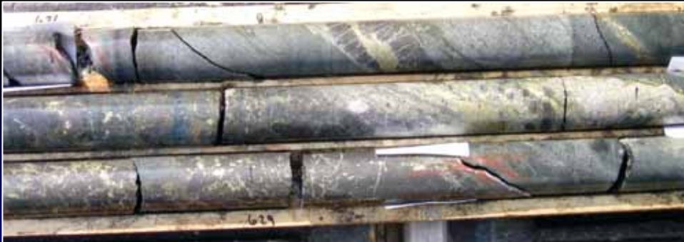
Veins and stringers of semi-massive magnetite and chalcopyrite containing visible gold
